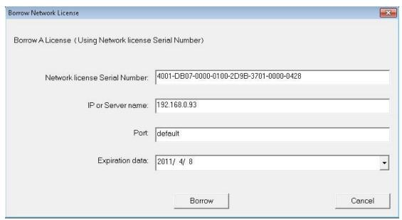
Click **Borrow**. Restart GstarCAD2011 and do not access to internet. Then GstarCAD2011 succeed to activate, and you can bring you computer to other place you want. However, the quantity of nodes is reduced until the borrowed one is to be returned.
