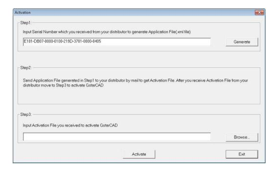
Click **Generate** to generate **Application File** and save it with a file name consisting of the **Serial Number** and ".xml" extension, e.g:
